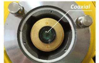
Coaxial Design of Tx/Rx Unit
