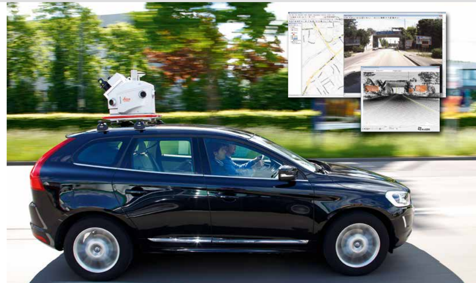
Leica Pegasus:Two combines the comfort and confidence of visual images with the accuracy of a point cloud at vehicle speed together into a GIS-enabled interface with semi-automatic extraction tools.
